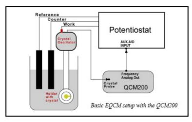
Fig. 2: EQCM and potentiostat, connection diagram
