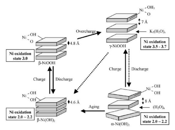
Fig. 1: Bode's diagram of Ni(OH)<sub>2</sub>
