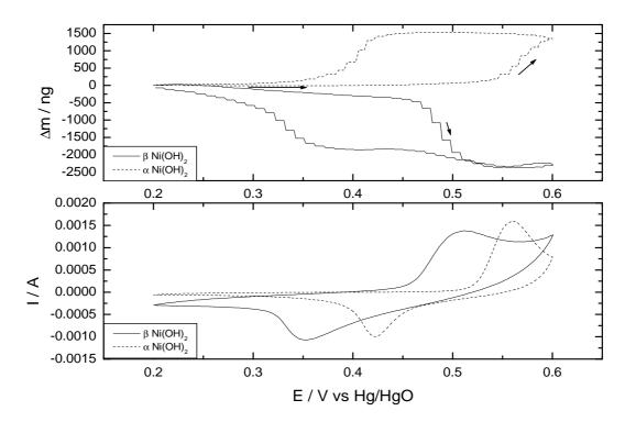
Fig. 3: CV and massograms of  $\beta$  and  $\alpha$  nickel hydroxides
